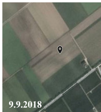
Figure 5-73. Example of the M7 false negative parcel. Due to the low NDVI values during most of the practice period (the practice period is marked in gray) the algorithm evaluates the vegetation as not growing while the interpretation of the Planet data indicates the vegetation was growing
