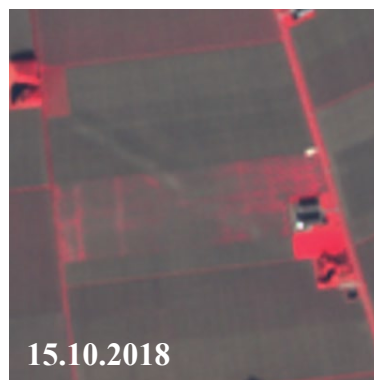
Figure 5-71. Example of the M6 false negative case. Due to low NDVI values within the practice period (marked in gray) the algorithm evaluated the vegetation as not present while the interpretation of the Planet data indicates the vegetation was present
