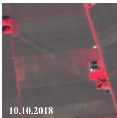
Figure 5-71. Example of the M6 false negative case. Due to low NDVI values within the practice period (marked in gray) the algorithm evaluated the vegetation as not present while the interpretation of the Planet data indicates the vegetation was present
