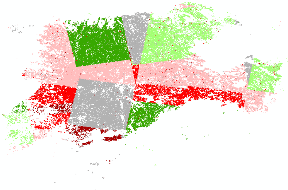
Figure 5-58. S1 data availability in CyL 2018 – The number of weeks for which the S1 data are completely missing is represented with a colour code: 8 – dark green, 9 – light green, 10 – pink, 11 – red, 12 – dark red, more than 12 weeks – gray
